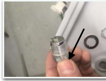
Remove the silicone pad from the bottom and top.
