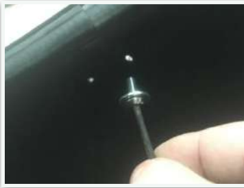
loosen the 3mm Imbus screws
