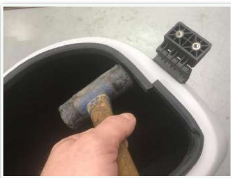
Installation of rubber seals
