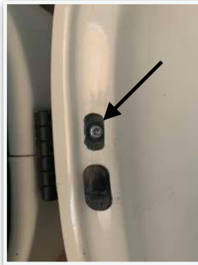
remove the 3mm Imbus screw
